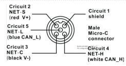
The NJ/JN GATEWAY works with Micro-C connector. The PIN layout is as follows:
