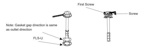
Step 2: Insert sensor into tank hole, tilt sensor, then insert one end lightly into tank opening
