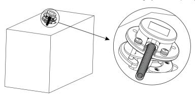
Step 3: Rotate sensor clockwise so it can rotate into tank
