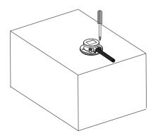
Step 5: Tighten screws firmly in star pattern
