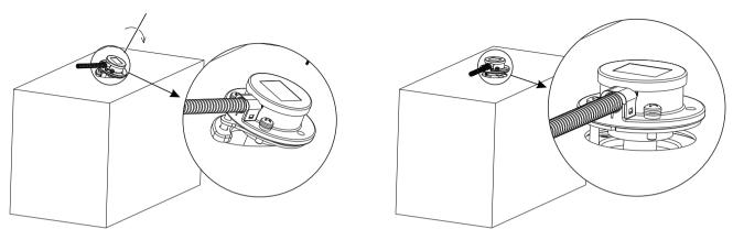
Step 4: Loosen screw, adjust FLS-U position, align other screws with screw hole on FLS-U, then tighten screws with screwdriver (do not lock).
