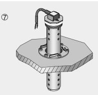
Thread the sender into the flange.
